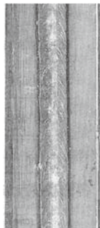
立向下進溶接
